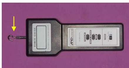
Fig.5 The measuring device in use. A hook for tension measurement (arrowed) is attached. Measurement values are displayed in digital presentation, and maximum value can be held in memory.
